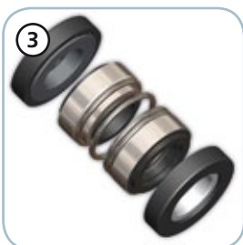
3 Mechanical seal Three mechanical seals; double seal (SiC-Al) in oil sump with food-grade oil lubrication, one V-ring in direct contact with the liquid.
