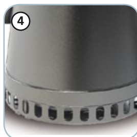
4 Strainer A special set allows the sewage pump to be transformed into a dry floor one. The minimum level of liquid can be lowered to 5 mm from the ground by setting two special shimming.
